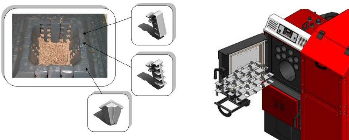
Figure 18. Display removing turbulators from boiler ECO COMFORT
